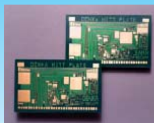
DENKA HITT PLATE (Al-base substrate(IMS))
